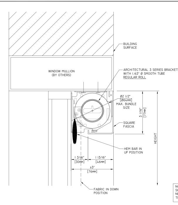
NOTE: SHIM MAY BE INSERTED IF NECESSARY TO PREVENT TELESCOPING.
