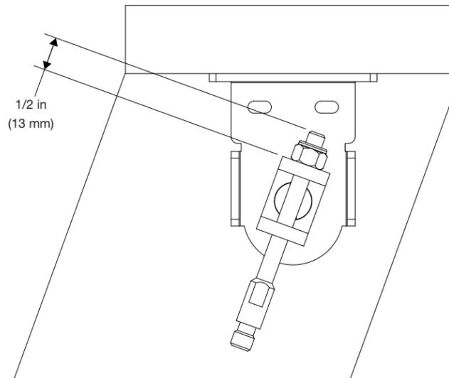
2. Feed the cable through the cable grip housing and then through the cable grip.
