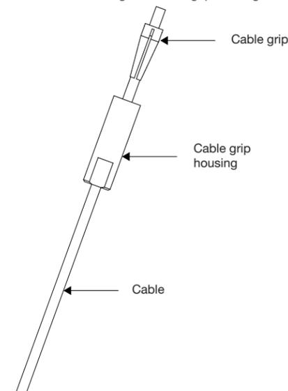
3. Bring the loose end of the cable to the top anchor and ensure that there is no slack in the cable. Using cable cutters capable of cutting 1/8 in (3 mm) stainless steel cable, cut the cable in line with the ridge indicated on the threaded rod. Slight fraying when the cable is cut is acceptable as long as the cable grip and cable grip housing can fit into the threaded rod.
