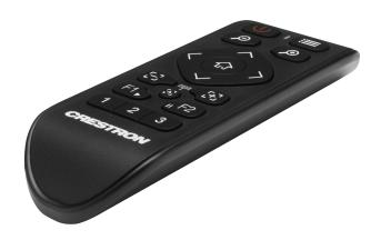
The IV-CAMA-REMOTE is an IR wireless remote designed to be used with IV-CAM-I12-B cameras. The IV-CAMA-REMOTE provides full access to camera video settings, calling predefined camera presets, and enabling or disabling camera tracking.
