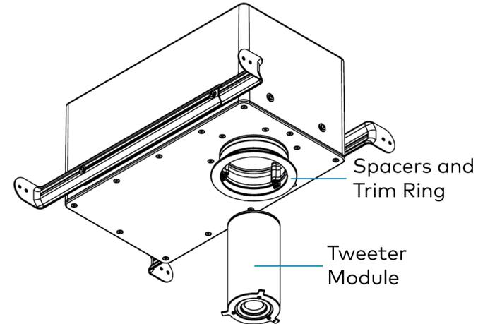
3. Rotate the tweeter module so its tabs slot into the trim ring tabs. Tighten the set screw located in one of the tabs on the trim ring using the included hex key.
