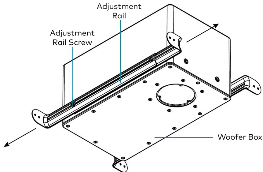
2. Using either the [SPKA-IC3-SA-MNT-TOOL](#) mounting bracket tool (sold separately) or spare two-by-four, create a temporary platform to hold the woofer box in place. Using a platform attached directly to the ceiling joists will ensure that the woofer box baffle is flush to the edges of the ceiling joists. If the woofer box is not flush with the joists, the ceiling material may not properly secure to the joists during installation, or it may bow outward.
