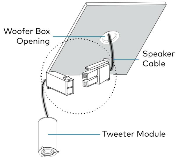
2. Fit the tweeter module through the trim ring and spacers into the woofer box opening.
