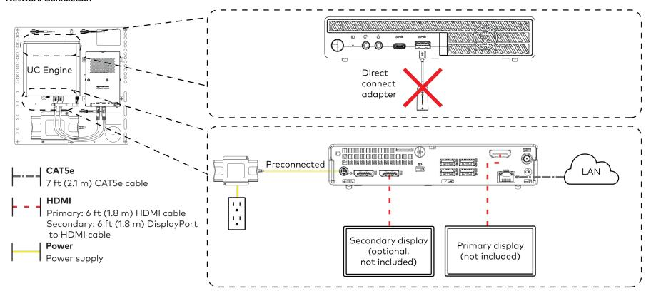
2. Make a network or direct connection on the bottom of the conference device as described in step 1. Make the remaining content ingest, laptop, mic pod, and power connections. Connect the conference device's power supply to an AC power outlet.
