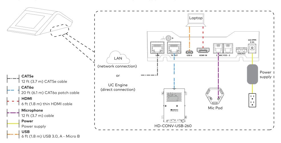
3. Connect the power supply and camera (not included) to the bottom of the content ingest device (HD-CONV-USB-260). Connect the power supplies to an AC power outlet.
