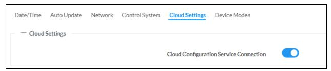
Set the **Cloud Settings** toggle to enabled (right) or disabled (left) to specify whether the DM-NAX-AUD-IO can communicate with the XiO Cloud® platform.
