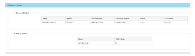
Occupancy sensors can be paired with the device using the **Occupancy Sensor** section of the **Settings** tab.
