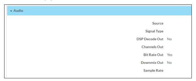
Information is only populated in this section for whichever audio input is selected as the active audio source. The active audio source is determined by the **Input / Output Selection** section of the **Settings** tab, or by commands issued by a control system.
