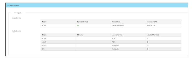
In the **Video Inputs** table, the **Sync Detected** status for the HDMI input displays whether or not a source is connected to the HDMI input. If sync is detected and a signal is passing, the **Resolution** and **Source HDCP** fields will also populate with information about the video signal.
