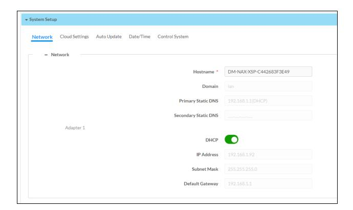
**NOTE:** By default, the hostname of the DM-NAX-XSP consists of the model name followed by the MAC address of the device. For example, DM-NAX-XSP-C442683F3E49.
