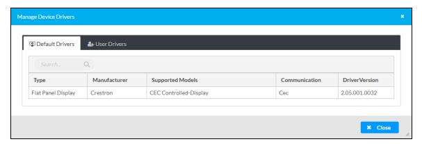
Click the Manage Device Drivers entry in the Action Menu to open the Manage Device Drivers window.
