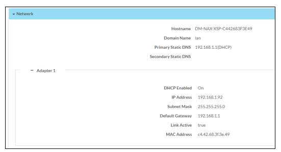
**NOTE:** By default, the host name of the DM-NAX-XSP consists of the model name followed by the MAC address of the device. For example, DM-NAX-XSP-C442683F3E49.
