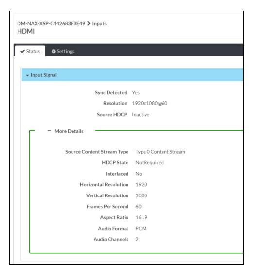
All four inputs have a read only **Status** tab that shows video and audio information for the connected source. Video status fields are only populated for the HDMI and eARC inputs, and will show **N/A** for the AES67 and BTS inputs.
