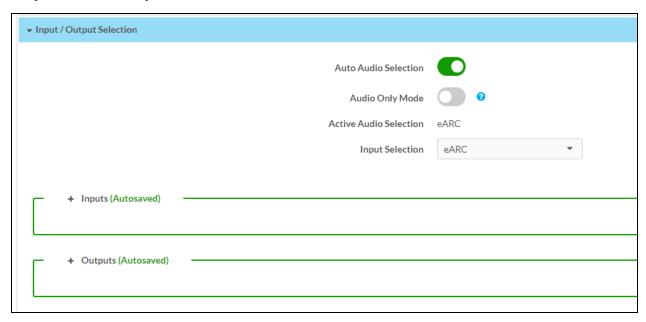
The **Auto Audio Selection** setting determines whether the active audio input of the DM-NAX-XSP is driven automatically by signal detection, or driven manually by either the **Input Selection** drop-down menu or programming.
