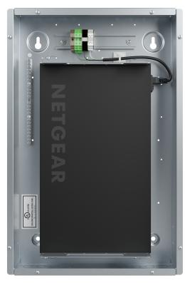
The Crestron® ZUML-SWPOE-26 is a preassembled lighting network expansion panel that expands Ethernet and Cresnet® network connectivity for a Crestron lighting system. It contains a CEN-SWPOE-26 26-port PoE+ switch mounted in a DIN-EN-3X18 wall mount enclosure.
